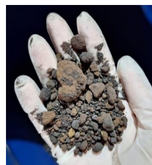
Figure 9. Product obtained after calcination for 24h under approximately 990°C. Source: authors.
